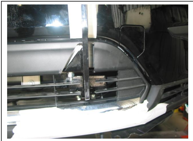
Figure 5: Cut out in plastic bumper with steel mounting bracket and grille fitted to vehicle
