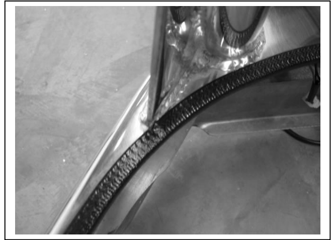
Figure 10: Clip lock beside tube gussets
