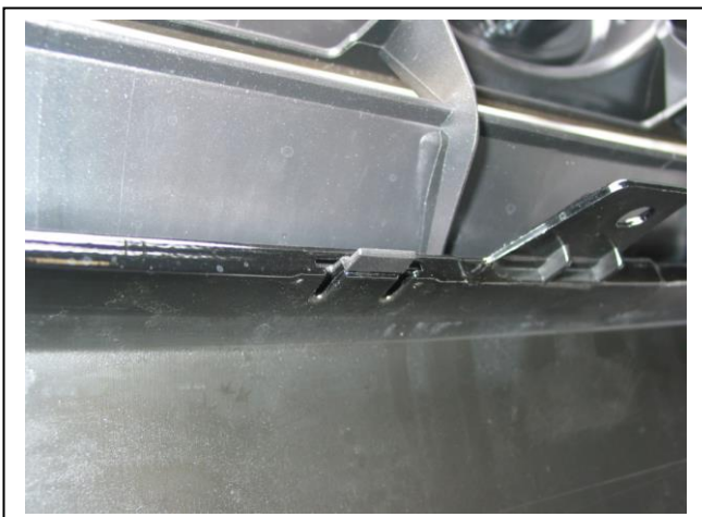
Figure 1: Lower view of grille clip. Push centre up
