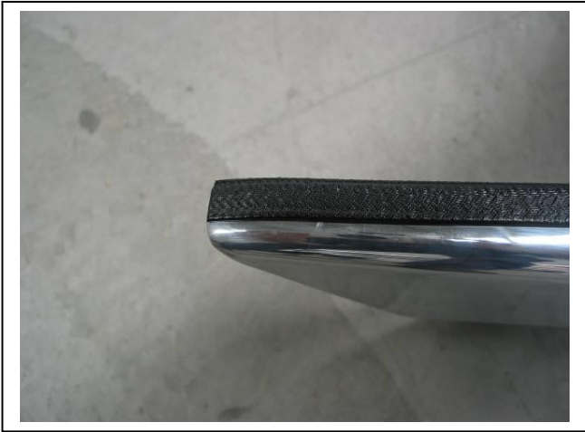
Figure 9: Cut end to match channel end
